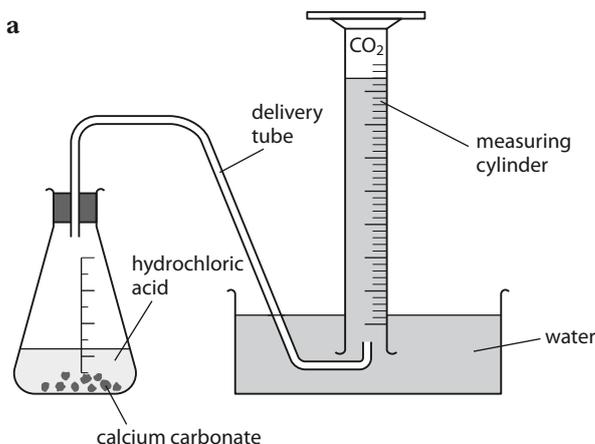
The volume of carbon dioxide produced is measured every 10 s.
